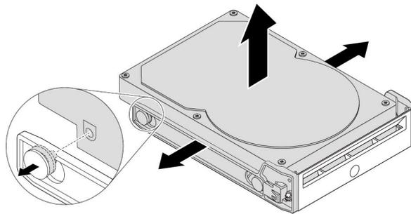
Figure 32. Removing the hard disk drive from the bracket
