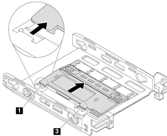
Figure 52. Pivoting the bracket
