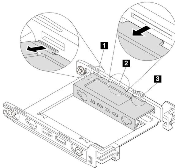
Figure 56. Releasing tabs **1**, **2**, and **3** from the corresponding slots
