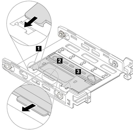
Figure 58. Inserting tabs **1** and **3** into the corresponding slots
