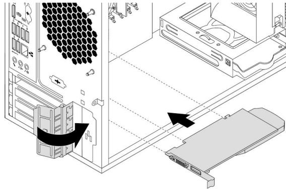
Figure 15. Installing a PCIe card
