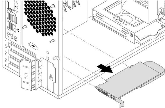
Figure 13. Removing a PCIe card
