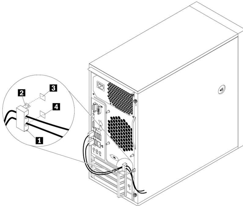
Figure 9. Installing a cable lock
