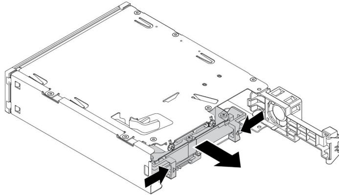
*Figure 46. Removing the 2.5-inch internal storage drive from the rear*
