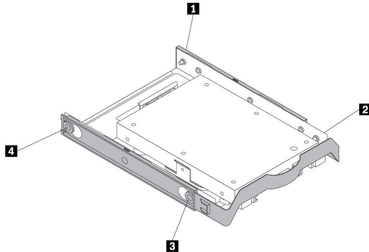
Figure 70. Installing the storage converter together with the solid-state drive into the storage drive bracket
