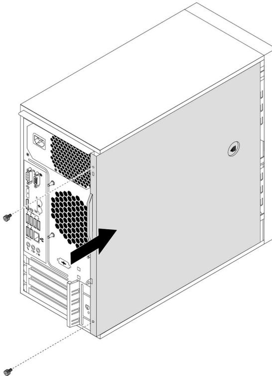
*Figure 79. Reinstalling the computer cover*
