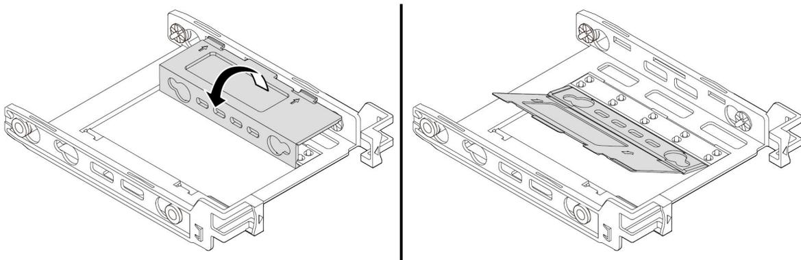
Figure 57. Unfolding the bracket
