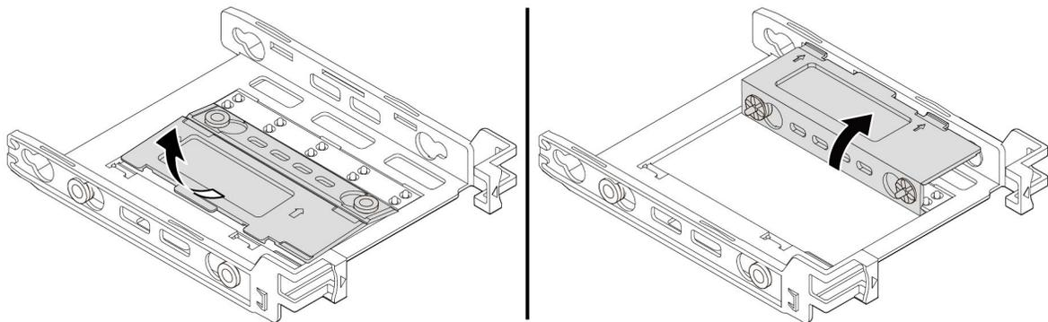
Figure 53. Folding the bracket
