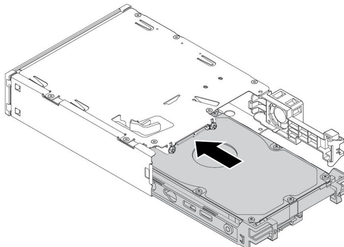
Figure 43. Sliding the new 3.5-inch internal storage drive into the kit
