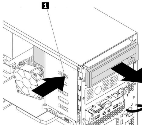
Figure 26. Removing the optical drive
