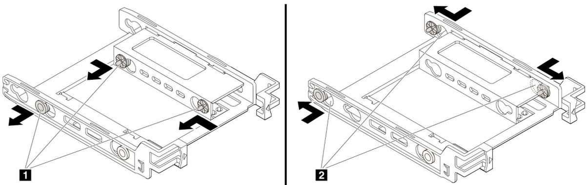
Figure 55. Removing three pins **1** and installing them into slots **2**
