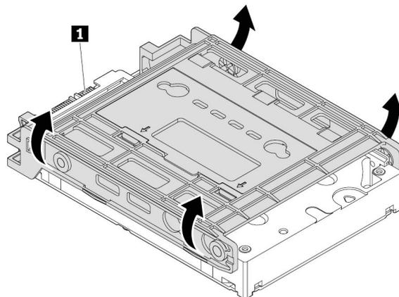
Figure 41. Flexing both sides of the bracket to remove the 3.5-inch internal storage drive
