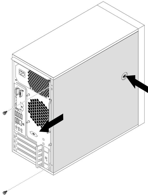
Figure 10. Removing the computer cover
