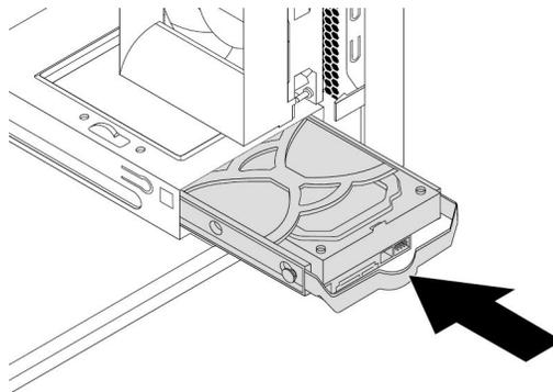
Figure 68. Installing the secondary hard disk drive
