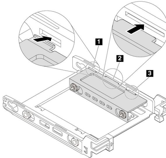
Figure 54. Inserting tabs **1** and **3** into the corresponding slots
