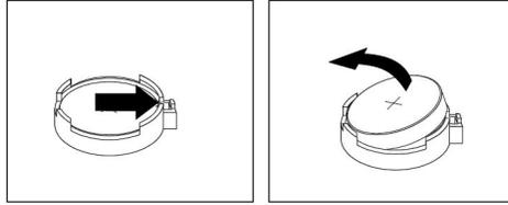
Figure 59. Removing the old battery
