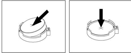
Figure 60. Installing a new battery
