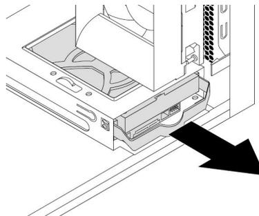
Figure 66. Removing the secondary hard disk drive
