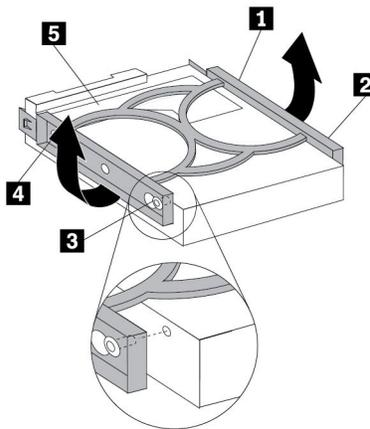
Figure 64. Installing the hard disk drive into the bracket
