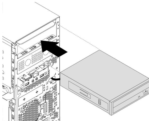
Figure 28. Installing the optical drive
