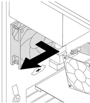
Figure 77. Removing the rear fan assembly
