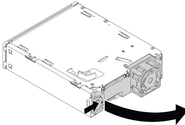
Figure 45. Opening the kit from the rear
