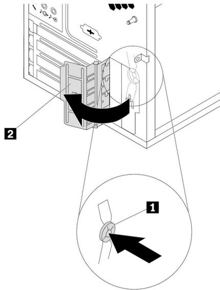
Figure 12. Opening the PCIe card latch
