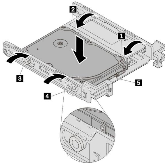
Figure 48. Installing the new 2.5-inch internal storage drive into the bracket
