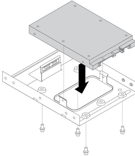
Figure 69. Installing the solid-state drive into the storage converter
