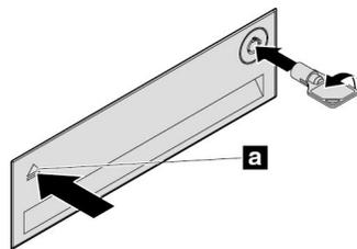
Figure 30. Opening the front-access storage enclosure cover
