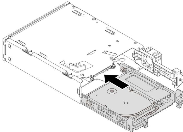
Figure 49. Sliding the new 2.5-inch internal storage drive into the kit
