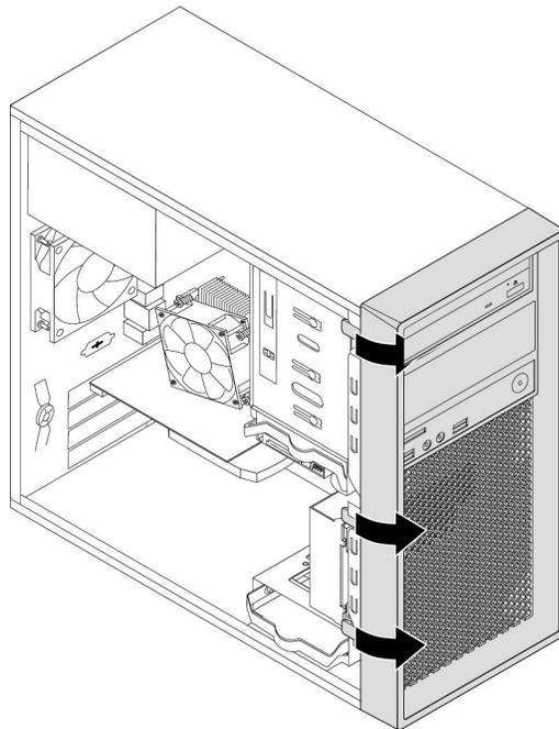
3. To reinstall the front bezel, align the three plastic tabs on the right side of the front bezel with the corresponding holes in the chassis. Then pivot the front bezel inwards until it snaps into position on the left side.
