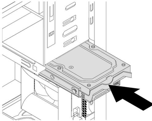
Figure 65. Installing the primary hard disk drive
