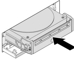
Figure 34. Installing the hard-disk-drive bracket
