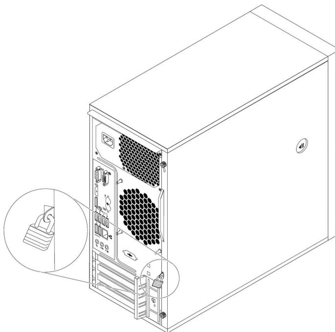
Figure 7. Installing a padlock
