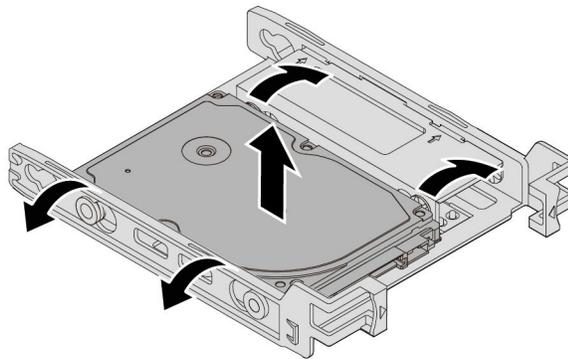
*Figure 47. Flexing both sides of the bracket to remove the 2.5-inch internal storage drive*
