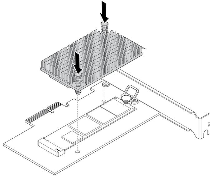
Figure 20. Installing the heat sink
