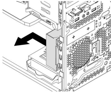
Figure 75. Removing the front fan assembly
