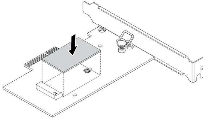
Figure 18. Installing the thermal pad
