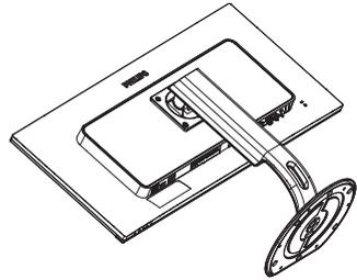
2. Loosen the assembly screws, then detach the neck from the monitor:
