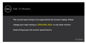
This means that the monitor cannot synchronize with the signal that it is receiving from the computer. See Monitor Specifications for the Horizontal and Vertical frequency ranges addressable by this monitor. Recommended mode is 2560 x 1440.
