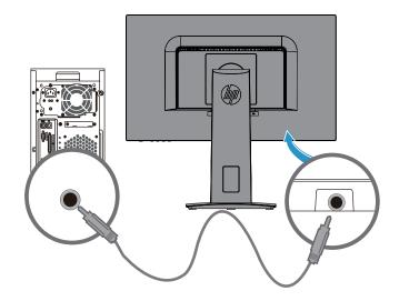
3. Connect one end of the power cord to the AC adapter (1), and the other end of the power cord to a grounded AC outlet (2). Then, connect the AC adapter to the monitor (3).
