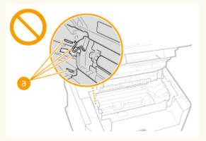
• Do not turn OFF the machine during printing. Also, do not open and close the cover and do not remove or insert paper during printing. Doing so can cause paper jams.
