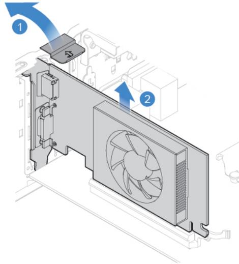
Figure 32. Removing a PCI Express card
