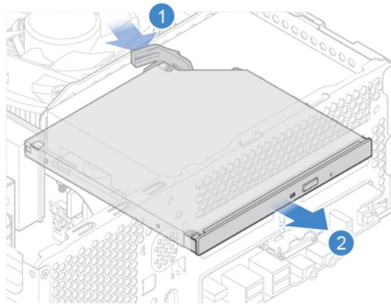
Figure 4. Removing the optical drive
