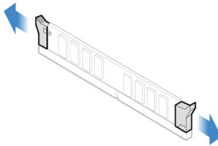
Figure 28. Disengaging the latches
