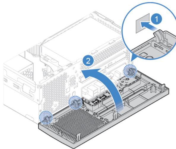
Figure 3. Installing the front bezel
