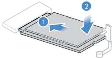
Figure 22. Installing the M.2 solid-state drive
