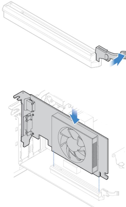
Figure 33. Installing a PCI Express card
