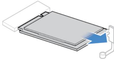
Figure 21. Removing the M.2 solid-state drive
