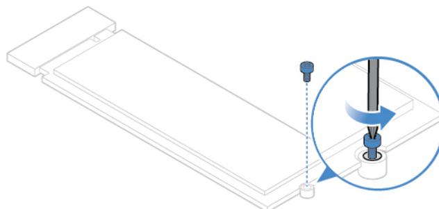
Figure 16. Removing the screw
