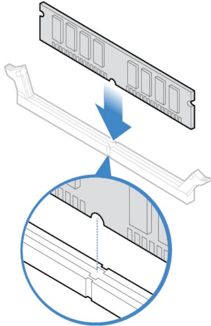
Figure 30. Installing a memory module
