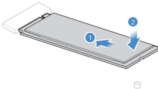
Figure 18. Installing the M.2 solid-state drive
