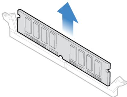
Figure 29. Removing a memory module
