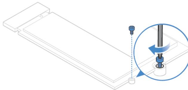
Figure 19. Installing the screw
