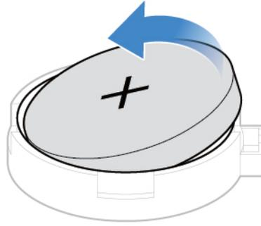
Figure 25. Removing the coin-cell battery
