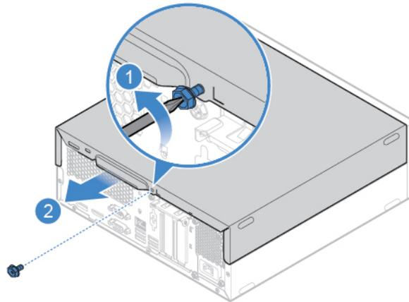
Figure 1. Removing the computer cover
