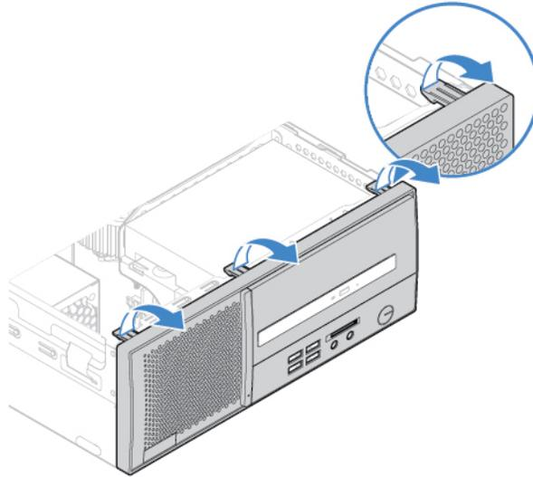
Figure 2. Removing the front bezel
