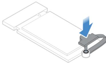
Figure 23. Inserting the stopper
