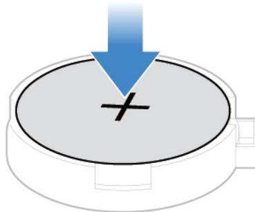
Figure 27. Securing the coin-cell battery with the latch
