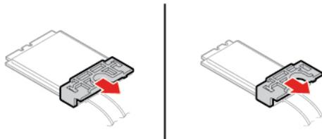
5. Disconnect the Wi-Fi antennas from the Wi-Fi card.
