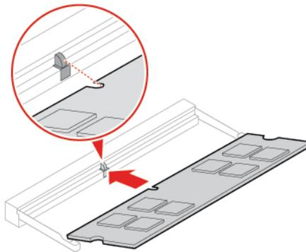
6. Secure the memory module with the latches.
