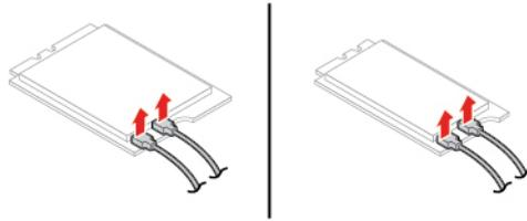
6. Connect the Wi-Fi antennas to the Wi-Fi card.
