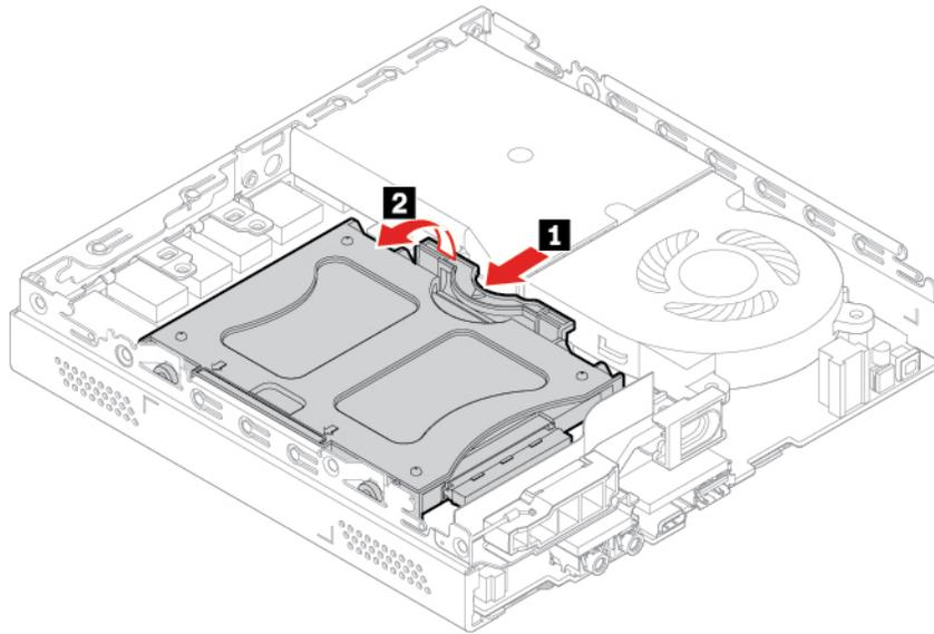
3. Disconnect the storage drive cable from the storage drive.
