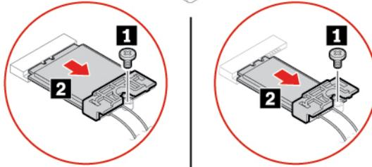
4. Remove the Wi-Fi card shield.
