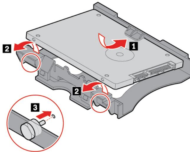
7. Turn over the storage drive so that the storage drive bracket is facing up.
