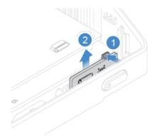
Figure 41. Removing the power button board
