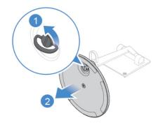
Figure 10. Removing the stand base from the stand bar
