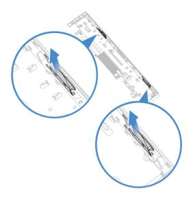
Figure 75. Removing the Wi-Fi antennas
