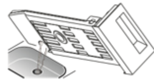
Slide out the water collection drawer
