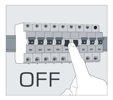
1. Ensure power is disconnected from the circuit and there is no risk of accidental reconnection before starting installation  Separate the Mounting Bracket (B) from the rear of the Ceiling Rose and fix in a suitable position on the ceiling adjacent to the supply cable using either the Screws (D) and Plugs (E) or using Bolts (C) into a suitable junction box. Care must be taken to ensure the mounting point is suitable for the weight of the fitting.
