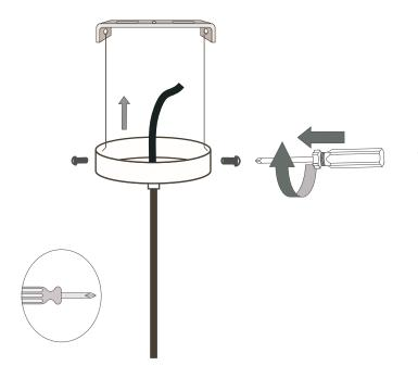
5. Reattach the Ceiling Rose to the Mounting Bracket using the bolts removed in Step 2.
