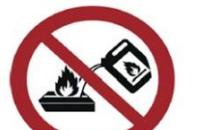
Do not fill fuel into the open flame or hot burner.
