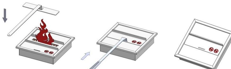
**NOTE:** Never extinguish the flame with water; let the fuel burn out completely if possible. This prevents alcohol from remaining in the reservoir and deflagration when reigniting.
