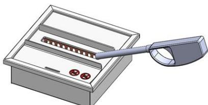
Use a long match or candle lighter to ignite the burner. Matches can be used, but you must ensure dead matches are not put into the burner.
