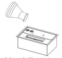
Any spilt ethanol must be immediately removed with absorbent tissue and cleaned with water to prevent ignition outside the burner reservoir.
